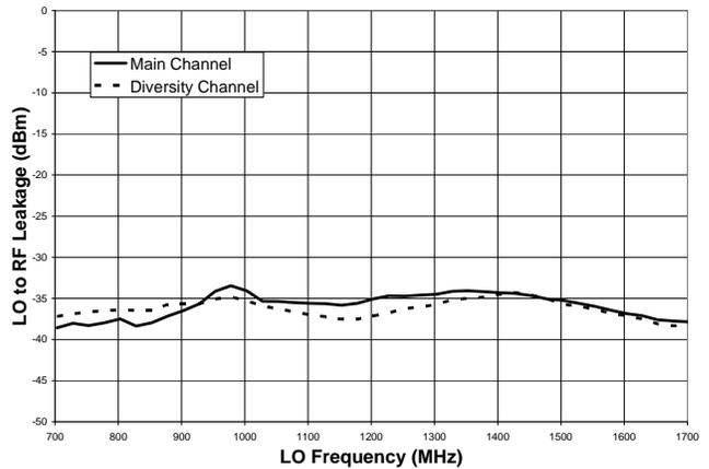
Figure 8. LO to RF Leakage versus LO Frequency
