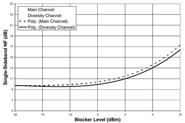
Figure 7. Single-Sideband NF versus Blocker Level at 1950MHz
