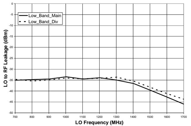
Figure 14. LO to RF Leakage versus LO Frequency
