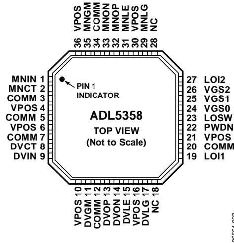
Figure 2. Pin Configuration
